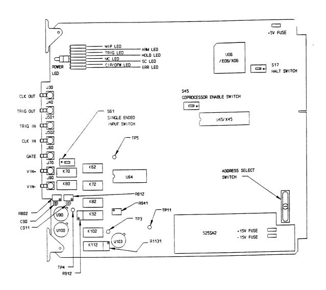
Figure 525-2: 53A-525 Card Assembly Drawing
