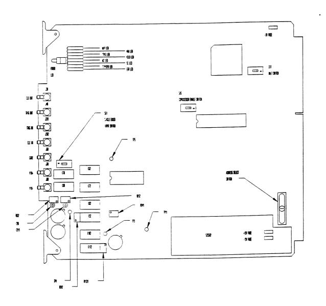
Figure 525-2: 53A-525 Card Assembly Drawing
